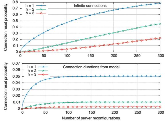
Figure 6. SHELL consistent hashing evaluation: probability for a connection started at time  $t = 0$  to be reset after  $n$  server reconfigurations.  $B = 35591$  buckets, 500 servers,  $c = 2$  choices, different history depths  $h$ . Top: infinite connections. Bottom: connection duration and server reconfiguration rate model from [13], [22].
