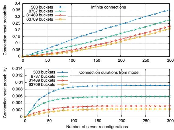
Figure 7. SHELL consistent hashing evaluation: probability for a connection started at time  $t = 0$  to be reset after  $n$  server reconfigurations. 500 servers,  $c = 2$  choices,  $h = 3$ , different number of buckets  $B$ . Top: infinite connections. Bottom: connection duration and server reconfiguration rate model from [13], [22].
