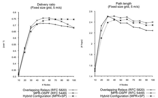
Fig. 9. (a) Delivery ratio and (b) path length (fixed size grid, 5 m/s).
