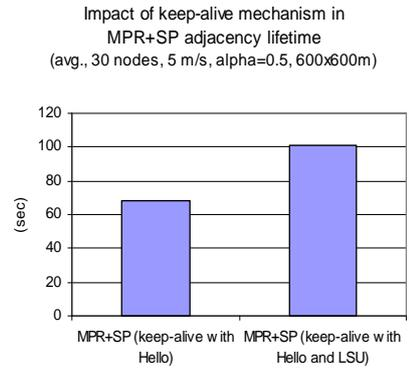
Fig. 14. OSPF keep-alive (*InactivityTimer*) impact in adjacency lifetime.
