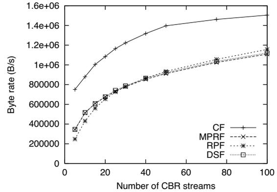
**Figure 2. Bandwidth Consumption for the four basic protocols.**
