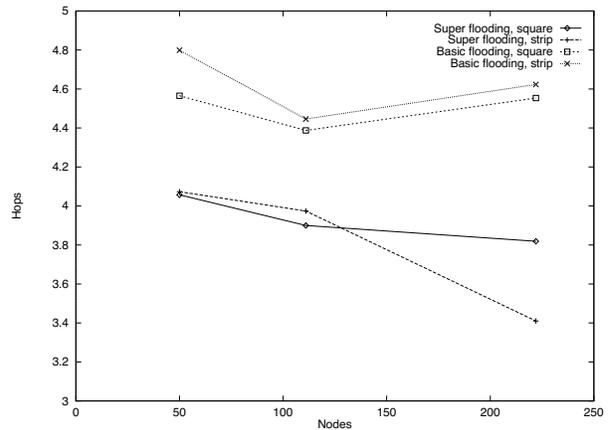
Fig. 13. Path length in a network with mobility.
