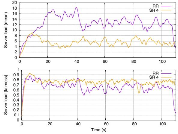
Figure 4. Instantaneous server load for a run of 20000 queries of the synthetic workload (mean and fairness over the 12 servers): Random vs  $SR_4$  policy,  $\rho = 0.88$
