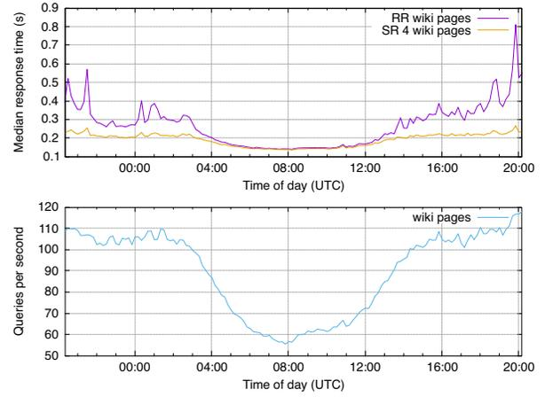
Figure 6. Wikipedia replay: query rate and median load time for wiki pages over 24 hours (10 mins bins). Random vs **SR<sub>4</sub>** policy.
