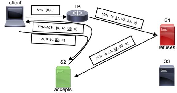
Figure 1. Service Hunting from client  $c$  to application  $a$  with 3 servers  $s_1, s_2, s_3$ . The path (source, segments, destination) is indicated between curly braces. The active segment is underlined.
