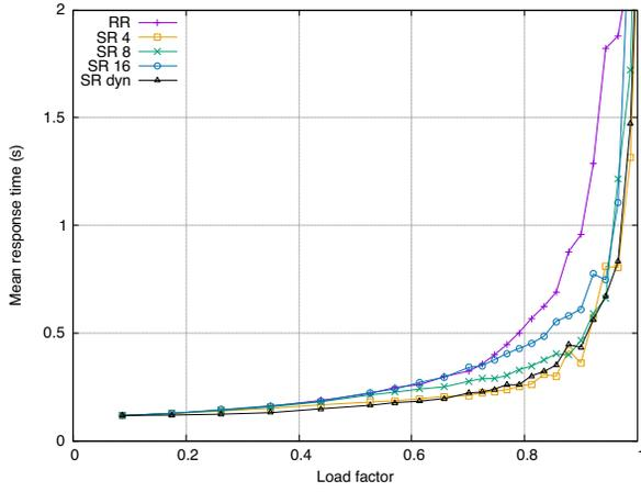
Figure 2. Average page load time for the synthetic workload: Random vs different  $SR_c$  policies (4, 8, 16, and dynamic). The dynamic threshold estimation closely follows the best policy (4 here)
